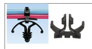
The Panduit THM1SC Harness Mount with a fir tree push barb holds wire bundles tightly and installs quickly into pre-drilled holes. The mount requires a panel hole diameter of .250" (6.5mm) and panel thickness between .03" to .14" (.9mm to 3.4mm). For use in indoor environments. Made of Nylon 6.6, these come colored as natural (not shown) or in Heat Stabilized black as shown. These come available in packs of 100 or 1000.
