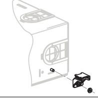
Attach strain relief clip with the #10-32 screw and nut provided.
