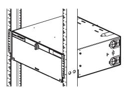
Bracket orientation for flush mount on a 19" rack Locate rack bracket on the front mounting holes for flush mounting.
