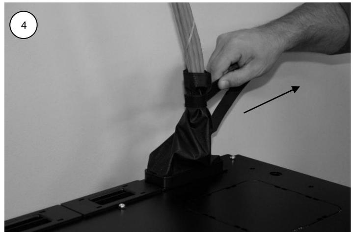
Step 4: Reattach the hook and loop at the top edge of the fabric sleeve. Pull the hook and loop cinch tie tight around the cable bundle. Wrap cinch tie around the cable bundle and attach it to itself. If applicable, trim off the excess cinch tie material.
