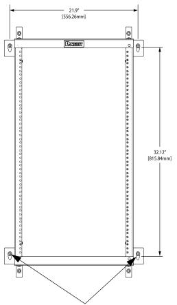
Keyhole mounting slots (.600"/ 15.24mm) allows for rapid, single-person instalation by pre-installing lag screws.
