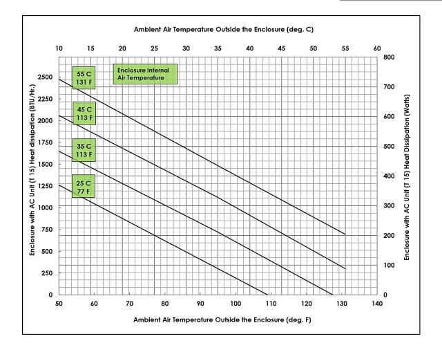
Figure 26: Z22 Enclosure Thermal Guideline – T15 Air Conditioner is available separately from Pentair. The outdoor model is equipped with a 150-watt heater. The maximum ambient operating temperature for the T15 is 55 °C. Therefore, the upper curves truncate at 55 °C outside ambient temperature.
