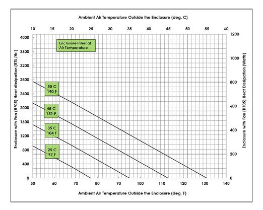
Figure 4: Z23 Enclosure Thermal Guideline – HF05 Fan Assisted. The HF05 Fan is available separately from Pentair.
