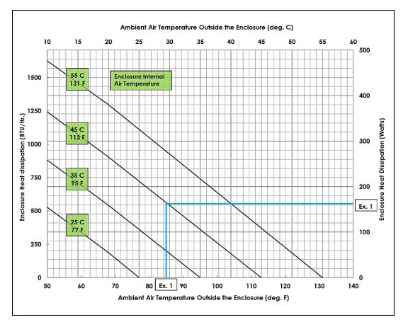
Figure 3: Z23 Enclosure Thermal Guideline – Sealed See next page for example situations and guidance for reading this chart
