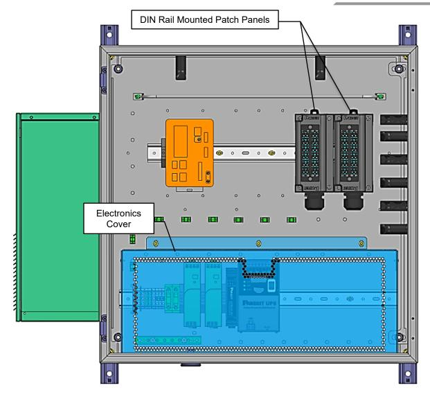
Figure 27: Front view of the Z22 Enclosure (front door removed for clarity).
