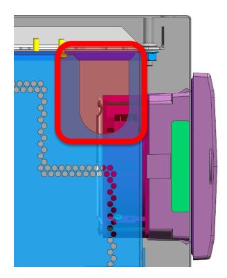
Figure 22: Z22 Enclosure with HF05 Fan installed on right (non-hinge) side. The area in red shows the reduced area for copper cable passing through the electronics cover with the fan mounted at this location.
