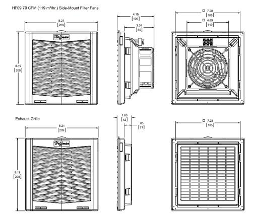
Figure 8: Dimensions of a HF09 exhaust fan and exhaust vent.
