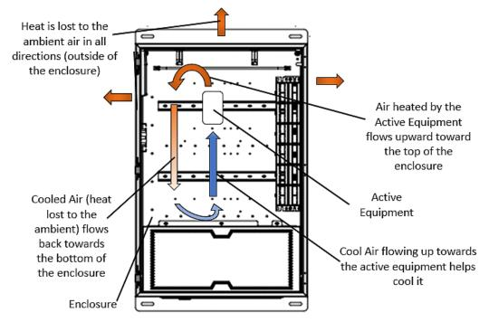
Figure 2: Idealized Thermal (aka Natural) Convection Cooling. Enclosure is 12" deep. The door has been removed to see inside the enclosure.
