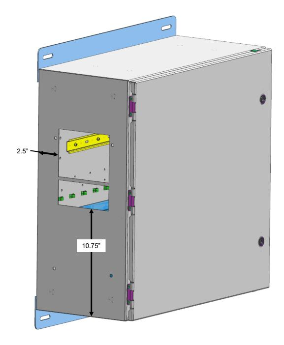
Figure 29: Shows the location of the cutout for the T15 AC unit on the Z22 enclosure. The cutout starts approximately 10.75 inches from the bottom of the enclosure and 2.5 inches from the rear of the enclosure.
