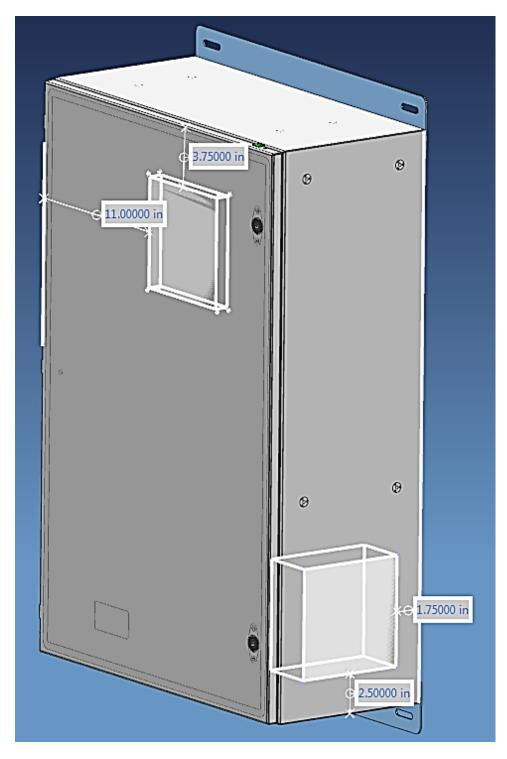
Figure 10: Approximate location for the HF09 fan and vent cutouts. The white lines give a relative indication of the space required for the fan and the dimensions show the location for the cutouts to install the fan and vent. The starting location is the same as the HF05 fan only the hole dimensions are larger. If desired, the fan can be installed on the opposite side of the enclosure, using the same positioning dimensions from the bottom & rear edges.
