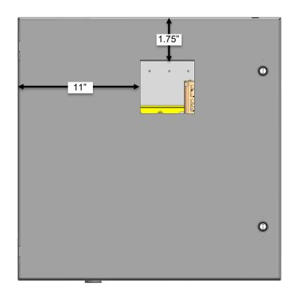
Figure 19: Z22 Enclosure HG05 Exhaust Opening Location. The HG05 Exhaust is available separately from Pentair.
