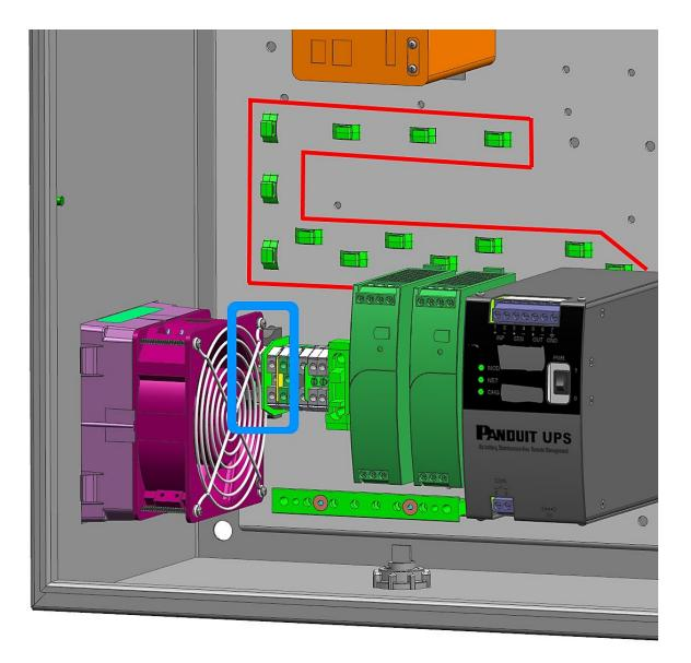
Figure 25: Z22 Enclosure with HF05 Fan installed on left (hinge) side. The area outlined in red shows where cable ties will need to be cut to make cable slack to slide the power supplies over. The area outlined in blue shows the terminal blocks that would interfere with the fan if not moved.
