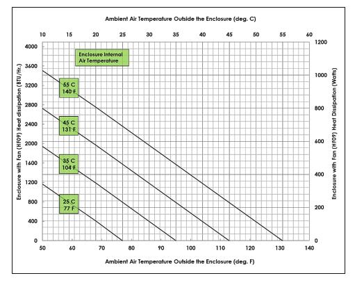
Figure 7: Z23 Enclosure Thermal Guideline – HF09 Fan Assisted. The HF09 Fan is available separately from Pentair.
