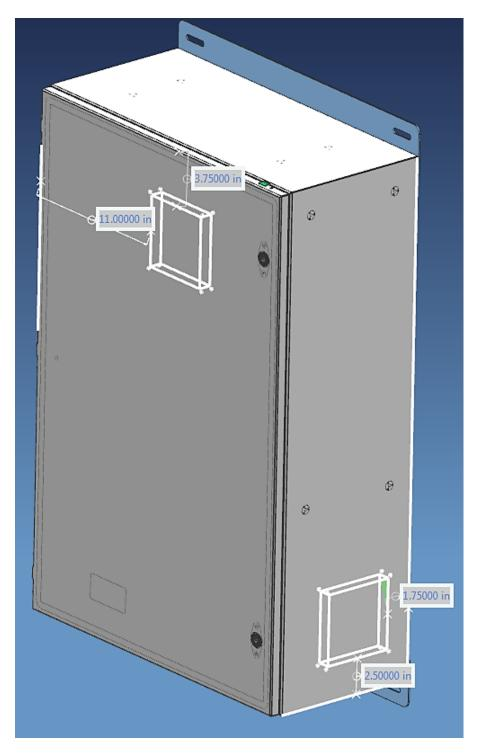
Figure 6: Approximate location for the HF05 fan and vent cutouts. The white lines give a relative indication of the location for the fan and the dimensions show the location for the cutouts to install the fan and vent. If desired, the fan can be installed on the opposite side of the enclosure, using the same positioning dimensions from the bottom & rear edges.
