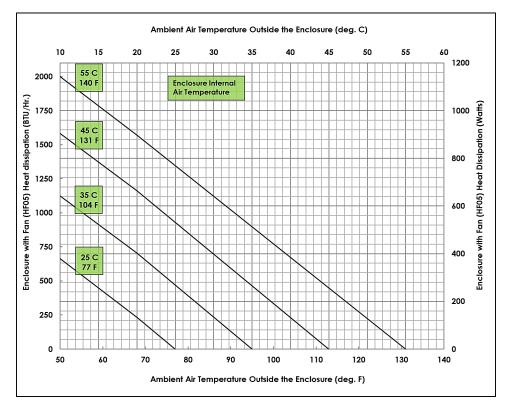
Figure 18: Z22 Enclosure Thermal Guideline – HF05 Fan Assisted. The HF05 Fan is available separately from Pentair.
