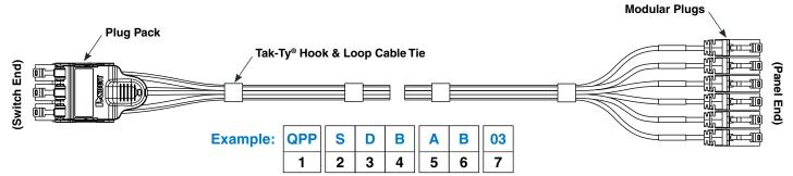
Part Number Example – QPPSDBAB03 is a 3-foot QuickNet<sup>™</sup> SD Switch Patching Harness with Category 6 UTP 28AWG CM/LSZH blue cable, a 6-position blue plug pack on one end, and modular plugs on the other end.
