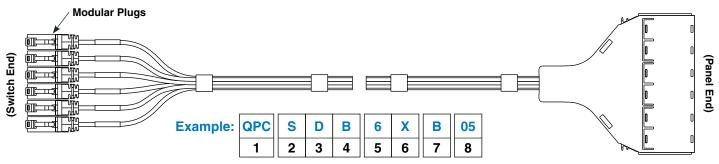
Part Number Example – QPCSDB6XB05 is a 5-foot QuickNet<sup>™</sup> SD Switch Port Harness with Category 6 UTP 28AWG CM/LSZH blue cable, modular plugs on one end, and cassette with blue modular jacks on the other end.
