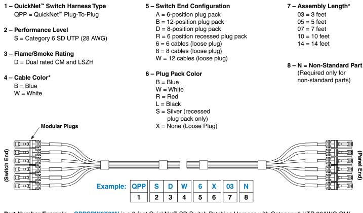
Part Number Example – QPPSDW6X03N is a 3-foot QuickNet<sup>™</sup> SD Switch Patching Harness with Category 6 UTP 28AWG CM/ LSZH white cable and modular plugs on both ends.
