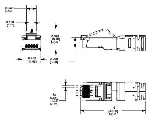
Dimensions are in inches. [Dimensions in brackets are metric].
