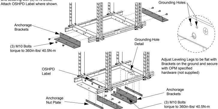
Note: If Anchorage Bracket covers grounding holes, Ground equipment using upper side to side beam grounding holes.
