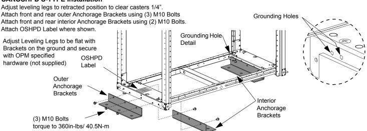
Note: If Anchorage Bracket covers grounding holes, Ground equipment using upper side to side beam grounding holes.
