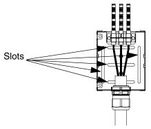
12.3 Power Distribution Unit Mounting Brackets - PEMS located on back of base accept #12-24 screws, which can be used to secure the breakout kit to PDU mounting brackets inside a cabinet.
