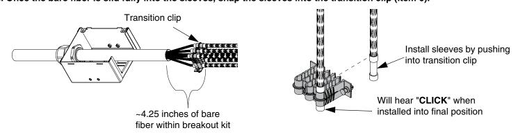
9. Once all sleeve assemblies are snapped into the transition clip (item 6), slide the base (item 1 or item 2) up the cable and snap the transition clip (item 6) into the base using the plungers and grommets.
