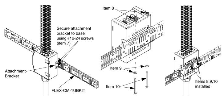
12.2 Bonus holes inside a cabinet - slots included on base allow for screws to be used to secure breakout kit base to holes.
