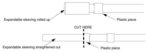
7. Feed the bare fiber groupings into sleeves (item 5). The sleeve will protect the bare fiber as it is being routed outside of the breakout kit and to the final location (splice tray, splice cassette, etc.).
