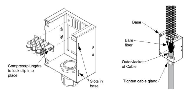
10. Lock down the cable in the base (item 1 or item 2) by tightening the cable gland.
