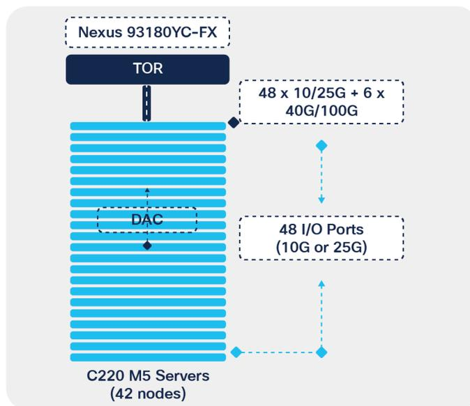
Figure 2. Server connectivity using 1 RU rack servers
