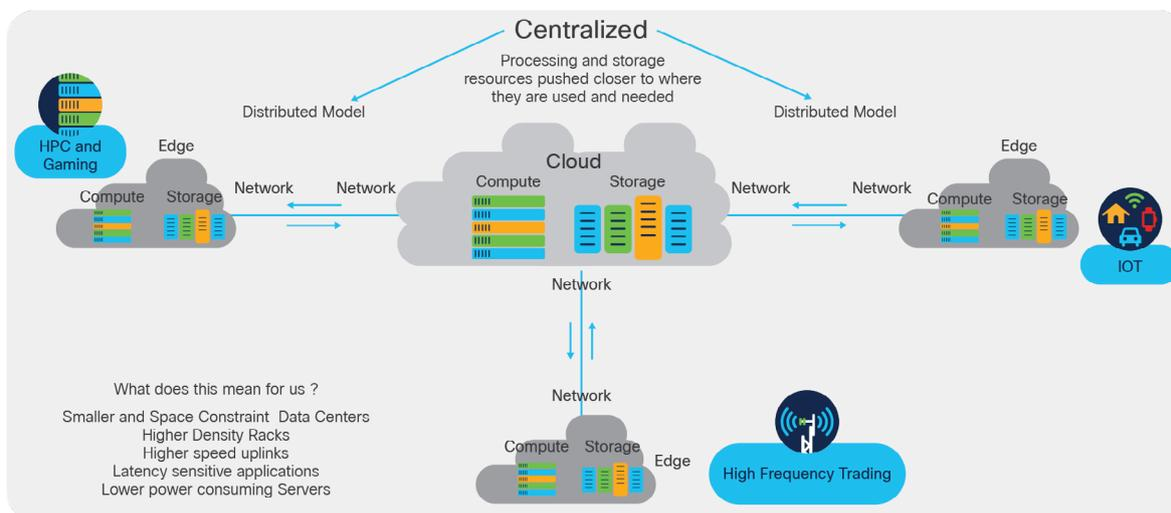
**Figure 1.** Transition from a centralized to a decentralized model for edge computing
