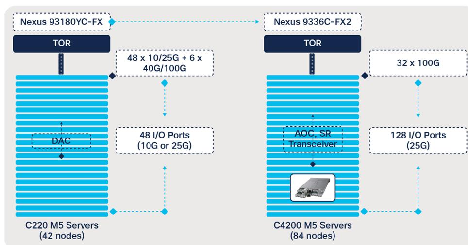
**Figure 3.** Rack density optimization using multimode chassis
