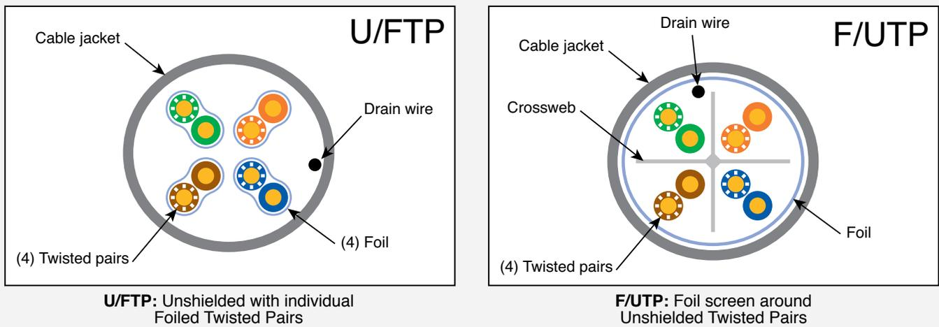
**U/FTP** and **F/UTP** are both shielded cables but are constructed differently. U/FTP has an unshielded jacket, with each individual pair wrapped in foil. F/UTP has a foil screen around the entire cable and each individual pair is not covered. F/UTP does have a crossweb to increase distance between the cable pairs.
