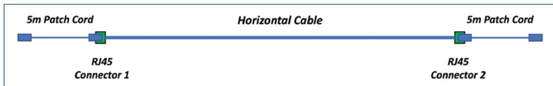
Figure 4: Representative Channel Configuration
