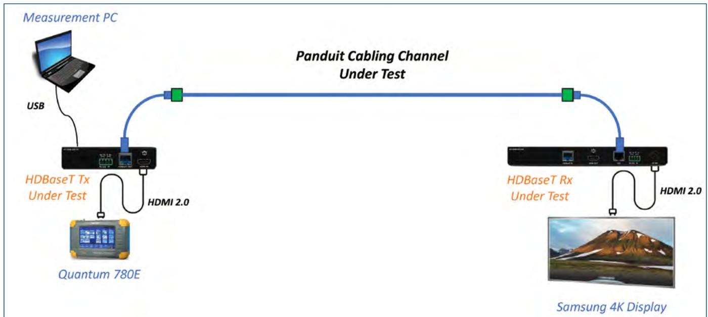
Figure 5: HDBaseT Performance Test Setup
