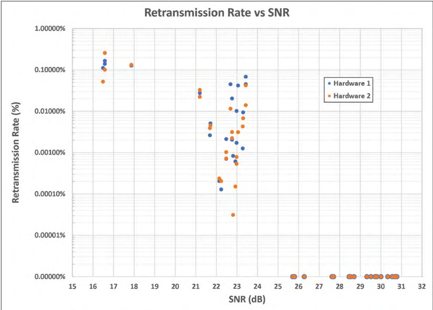
Figure 7: Packet Retransmission Rate vs SNR
