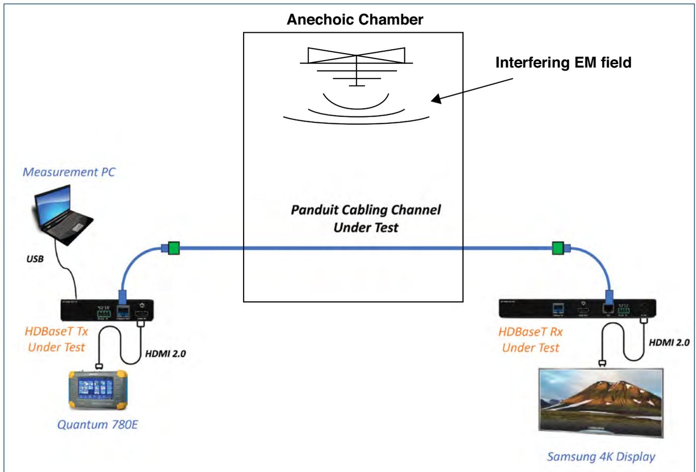
Figure 10: Electromagnetic Interference Test Setup
