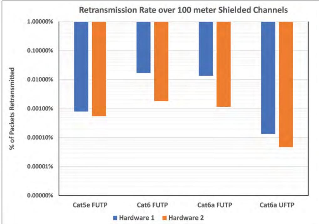
Figure 15: Retransmission Rate Measured over 100m Shielded Channels
