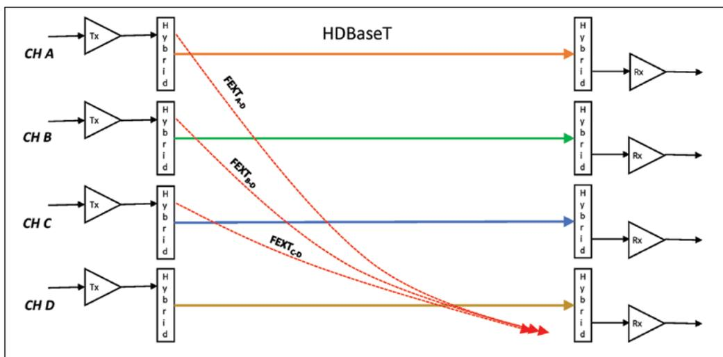
**Figure 2: HDBaseT Noise Impairments from Cabling Channel**
