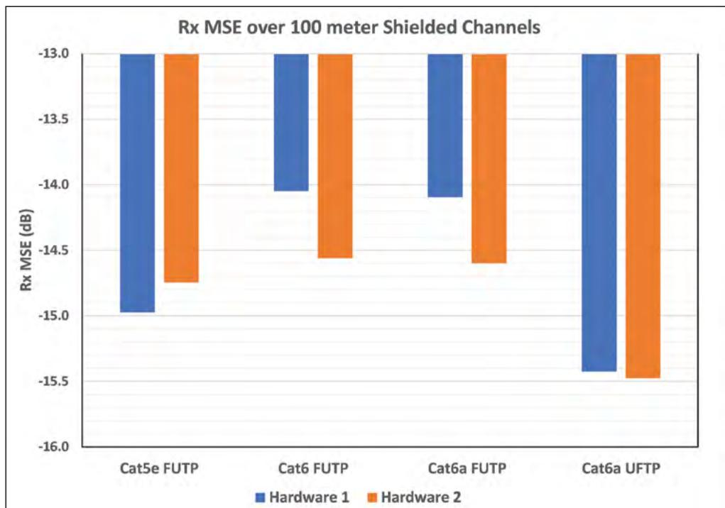
Figure 14: Rx MSE Measured over 100m Shielded Channels
