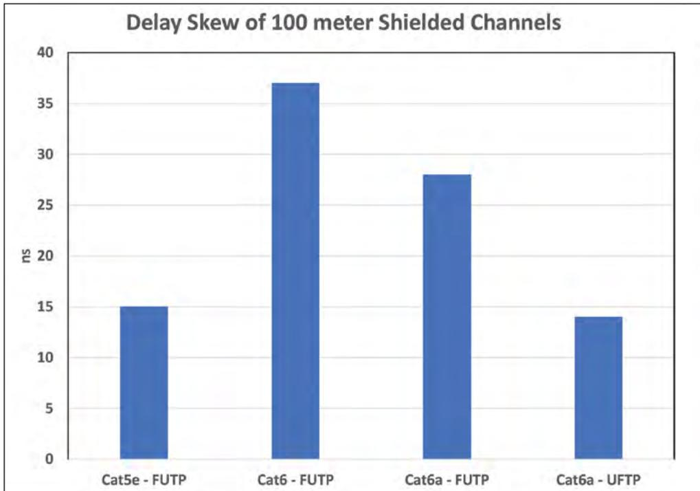
Figure 13: Delay Skew of Shielded Cabling Channels
