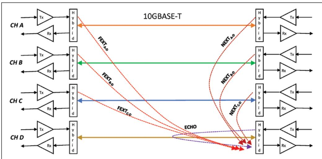
Figure 1: 10GBASE-T Noise Impairments from Cabling Channel
