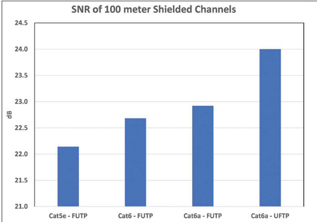
Figure 12: SNR of Shielded Cabling Channels
