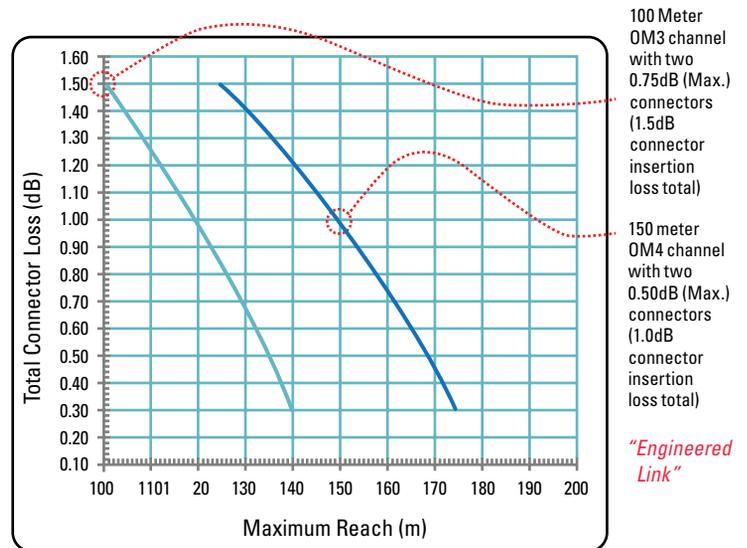
**FIGURE 3:** Extrapolation/interpolation from IEEE model for various connector insertion loss values.
