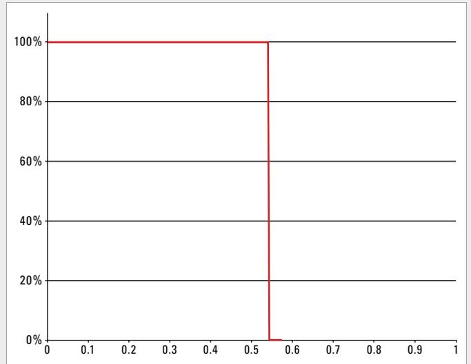
Measurement system should reject any links above 0.54 dB and pass all links below 0.54 dB. It will not create any false fails or negatives in the process.
