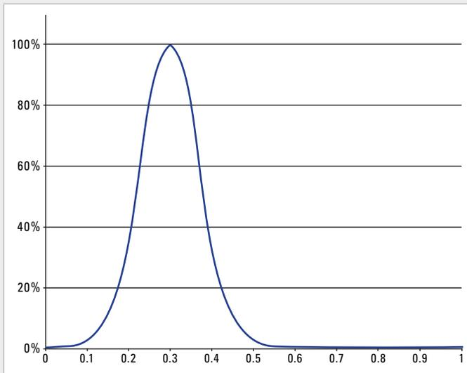
Here an artificial distribution of link losses that represent the “real” results if large numbers of such links were measured as in a lab environment.
