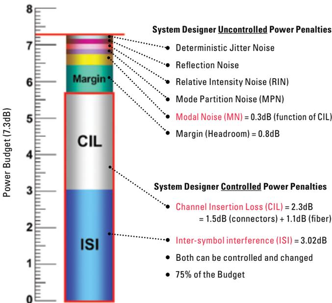
**FIGURE 1:** Optical channel budget for 10 Gb/s Ethernet trade-off parameters.
