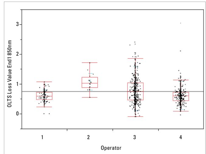
**FIGURE 11:** Box-Whisker chart of fan-out insertion loss versus operator measuring the same product.
