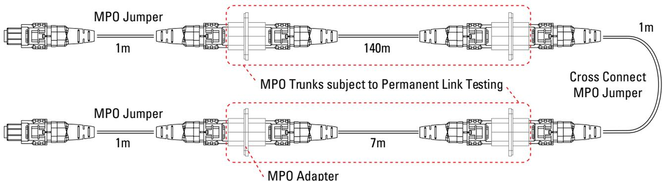
**FIGURE 4:** Parallel optics cross-connect cable plant.
