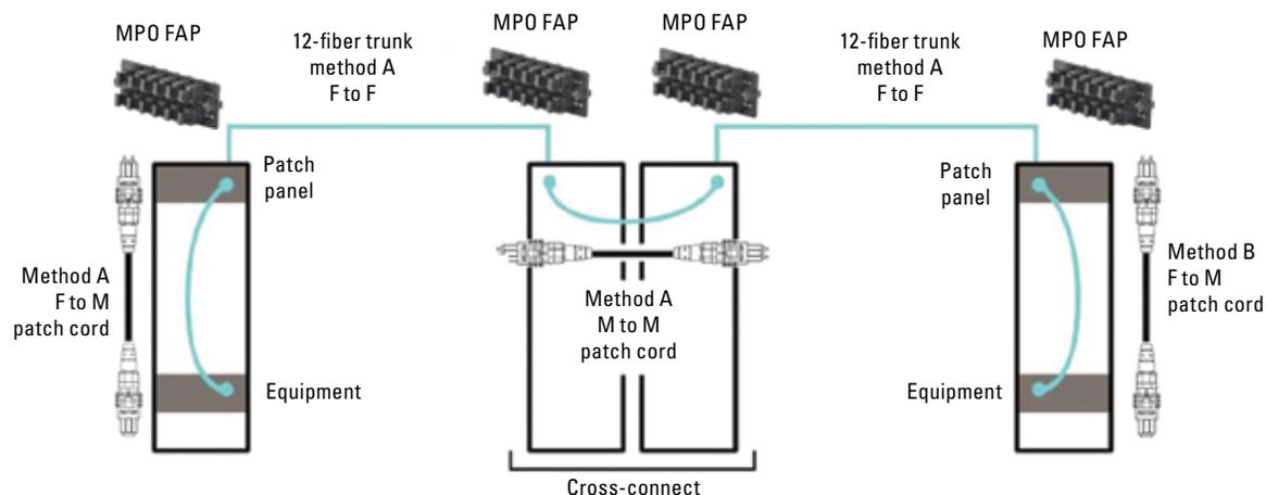
**FIGURE 2:** 40GBASE-SR4 engineered channel example.
