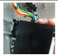
4. Snap the Isolation Module on the DIN rail. Alternately, the Isolation Module can be mounted to any surface using three, #8 pan head screws or another compatible fastener. Surface mounting with screws is recommended for high-vibration environments.
