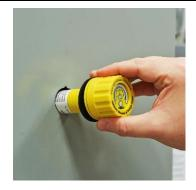
Insert the Indicator Module in the 30mm knockout hole, align antirotation notch. Ensure the rubber washer is on the outside of the enclosure.
