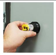
3. Tighten the panel nut until both it and the sealing washer make full contact with the enclosure surface. Then, tighten an additional ¼ turn. Tighten the panel nut with fingers only, do not overtighten.
