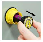
Grip the battery tray and slide it out until you feel a stop. The battery tray is not intended to be fully removed.
