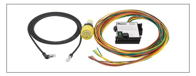
The VeriSafe Absence of Voltage Tester is a permanently-mounted tester that is used to verify a circuit is deenergized prior to opening an electrical enclosure. Once installed, a push of a button enables qualified electrical workers to verify the absence of voltage and see an active indication when the absence of voltage is confirmed. The Indicator Module is designed for a 30-mm notched panel knockout and the Isolation Module can be mounted to DIN rail or surface mounted using screws.
