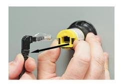
Continue holding the Retention Spring down while pulling back on the right-angle connector to release the AVT System Cable.
