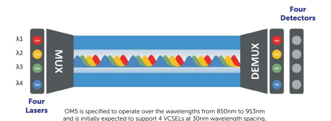
In the above example, four wavelengths of light each transmit 25Gbps resulting in 100Gbps across a single fiber, and full transmit (Tx) / receive (Rx) over a pair of fibers (as opposed to previous generation 100Gpbs standards that required many fibers or parallel optics). This concept can be applied to OM3, OM4 and OM5 fiber grades.
