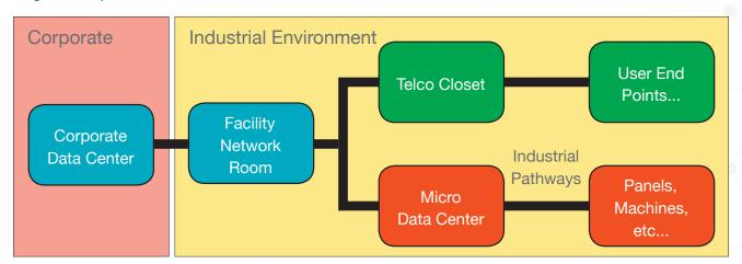
Figure 3. Block Diagram Indicating Location of Micro Data Center in Relation to the Data Center, Corp Network, Industrial Pathways, and Equipment Panels
