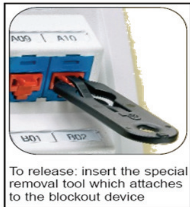
Figure 2.8-5. Example Blockout Device to Support Network Security Initiatives at Control Panel Locations
