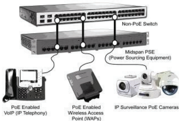
Figure 4.10-1. Applications currently driving the adoption of PoE include Voice over Internet Protocol (VoIP) phones, wireless access points (WAPs), and IP security and surveillance cameras.
