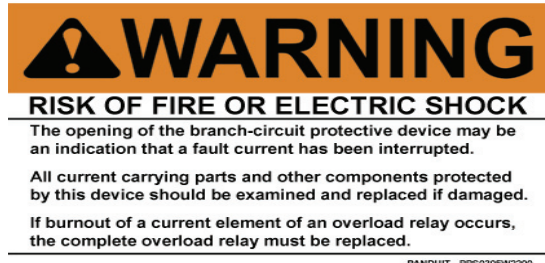
UL 508A Warning Sign
