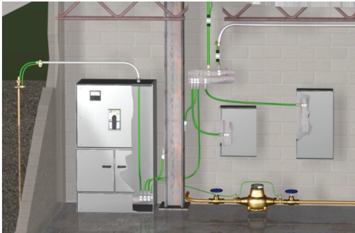
Figure C-1 – Service Entrance Grounding
