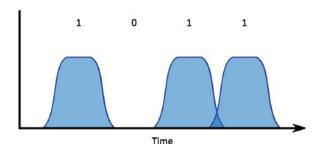
Eventually, as the distance lengthens or the speed of the pulses increase, e.g., 10G to 40G Ethernet, the effects of dispersion make it difficult and nearly impossible to distinguish the individual pulses.
