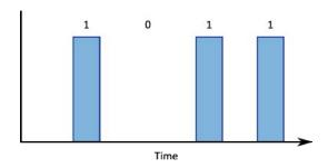
When the pulses emerge from the fiber at the other end, they are distorted as a result of modal and chromatic dispersion.
