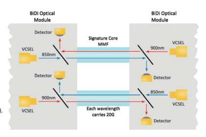
40G Ethernet BiDi optical modules are able to support 40G over 2 fibers because it uses two lasers, with different wavelengths (850nm and 900nm), pointing in opposite directions. The lasers run at 20 Gbps for a total bandwidth of 40 Gbps.
