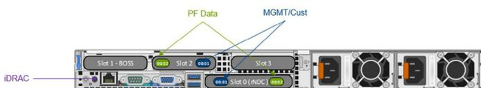
A PowerFlex R640 Appliance is used as a basis of design in this infrastructure. Deployment in a rack should be grouped with no more than 8 continuous rack units without a thermal break. The Cisco 93240YC-FX2 can support a total of 24 Nodes utilizing the configuration shown. Out of Band services will be handled with the Nexus 92348GC-X platform. Nodes will be deployed in a bottom-up fashion as the stack grows.
