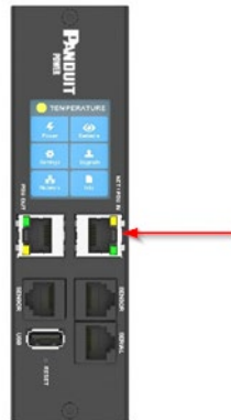
Figure 2: Ethernet Port for Network Connection
