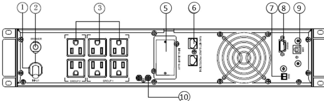
**Figure 7: 1.5kVA Li NA Rear Panel View (U02x11L)**
