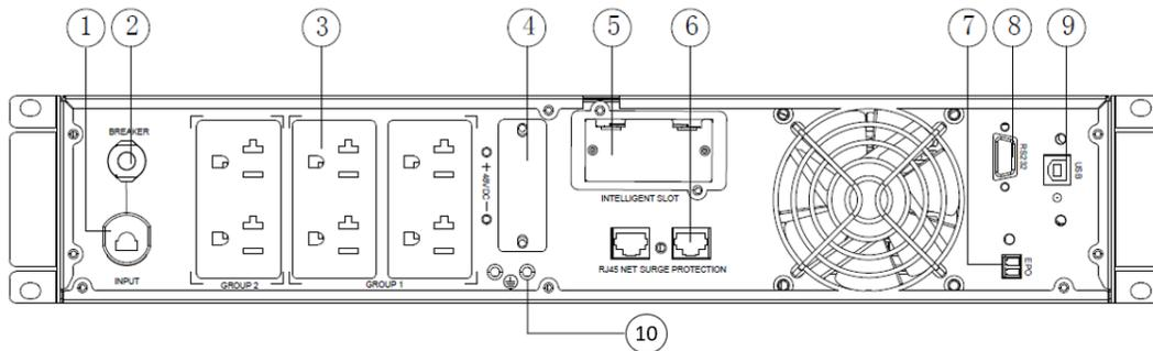
**Figure 6: 2kVA VRLA NA Rear Panel View (U02x11V)**
