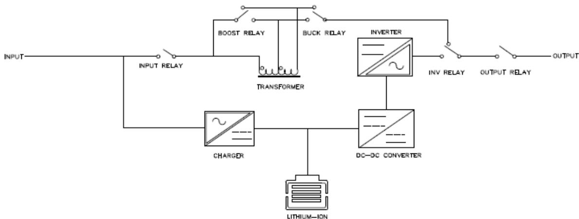
**Figure 2: High-Level Generic Line Interactive UPS Block Diagram**
