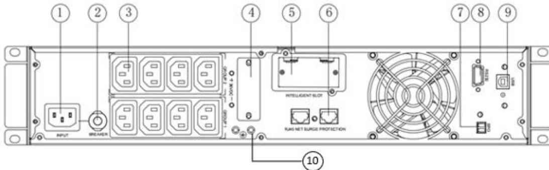
**Figure 10: 1kVA VLR/Li EU Rear Panel View**
