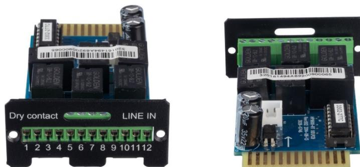
**Figure 14: Relay Card Front and Top View (showing connection points)**
