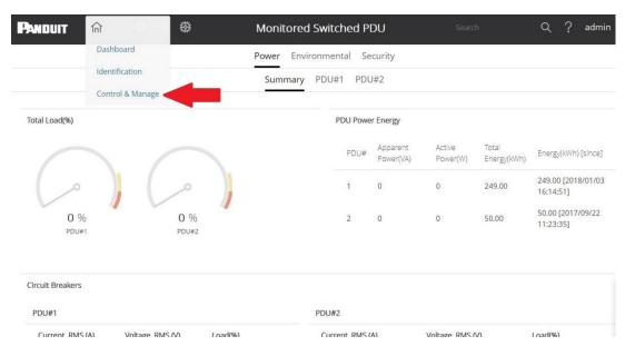
Figure 49: Control & Manage PDU
