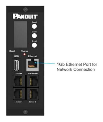
Figure 1: Ethernet Port for Network Connection
