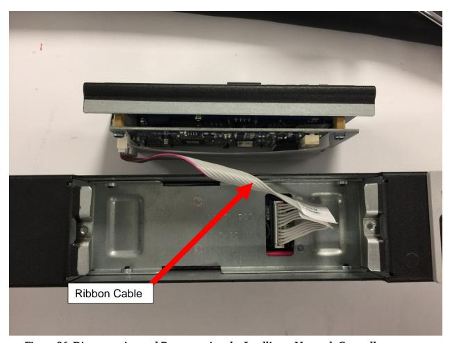
Figure 86: Disconnecting and Reconnecting the Intelligent Network Controller
