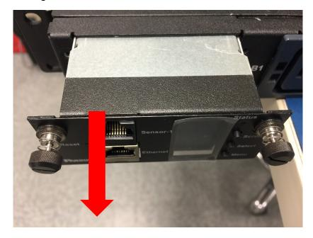
Figure 83: Remove Intelligent Network Controller from PDU
