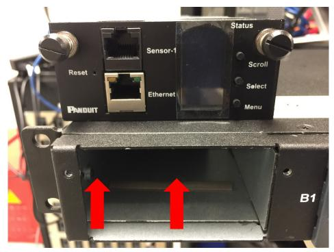
Figure 84: Inserting New Intelligent Network Controller
