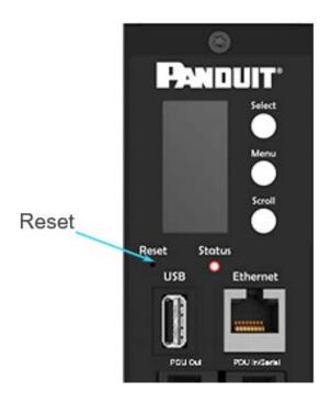
Figure 2: Locate Reset Button
