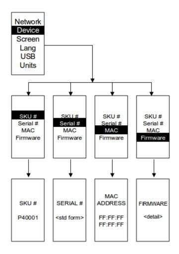
Figure 28: Device Submenu
