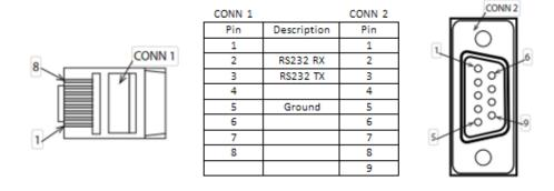
Figure 22: Serial Cable Pinout
