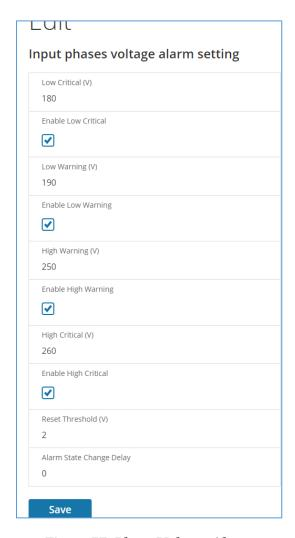
Figure 57: Phase Voltage Alarm
