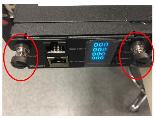
Figure 82: Unscrew Intelligent Network Controller
