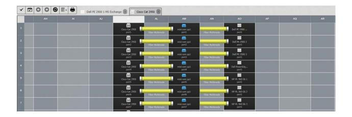
As part of the SmartZone Software Suite, SZ-Connect enables data center managers to build and view end-to-end connectivity of IT network devices. SZ-Connect provides the ability to capture the capacity of switches, utilization, and availability of switch ports. When paired with PViQ<sup>TM</sup> Patch Panels, PViQ<sup>TM</sup> Patch Cords, and Intelligence Modules, guided moves, adds and changes, and guided patch cord tracing will be provided throughout the network.
