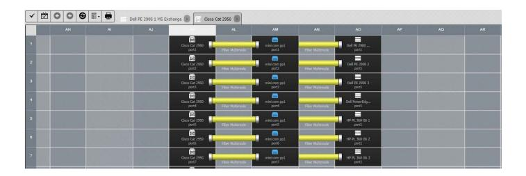
As part of the SmartZone Software Suite, SZ-Connect enables data center managers to build and view end-to-end connectivity of IT network devices. SZ-Connect provides the ability to capture the capacity of switches and utilization and availability of switch ports. When used with PViQ<sup>™</sup> Patch Panels, Intelligence Modules, and PViQ<sup>™</sup> Patch Cords, this SZ-Connect provides guided moves, adds and changes, as well as guided patch cord tracing.
