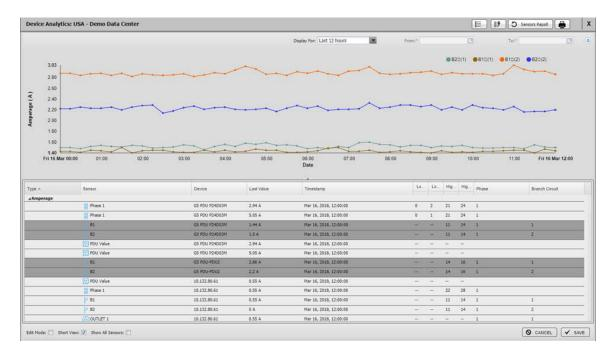
SmartZone™ Power provides users a wholistic view of where power and energy is consumed. Provides data center managers the ability to view the consumption of power and measures how efficiently the data center is utilizing power. Real-time events and notifications based on user defined thresholds are available along with current and volt consumption. Users can view the impact on power capacity and have at-a-glance views of PDU's analytics.
