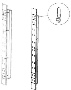
2. Install the PDU using the bracket mounting buttons and the mounting brackets located at either end of the PDU.
