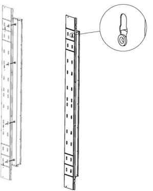
2. Install the PDU using the bracket mounting buttons and the mounting brackets located at either end of the PDU.
