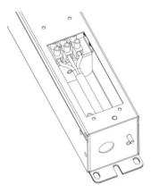
3. Ensure that the cover is replaced and secure before commissioning.
