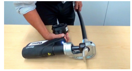
6. After the compression is over, the tool head will automatically return.
