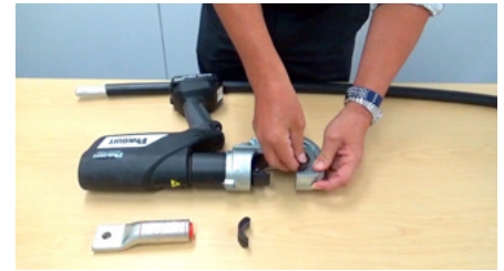
3. Install the die on the tool head.
