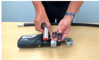
2. The part number printed on the terminal is the same as the die number.
