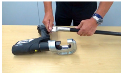
5. The 240 mm 2 terminal is compressed 4 times.
