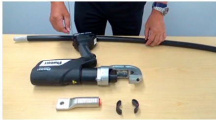
1. Prepare terminals, dies, tools and cables.
