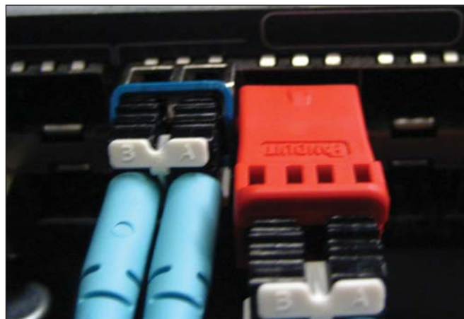
Figure 3. LCTRDC meets SFQ Transceiver MSA Specification
