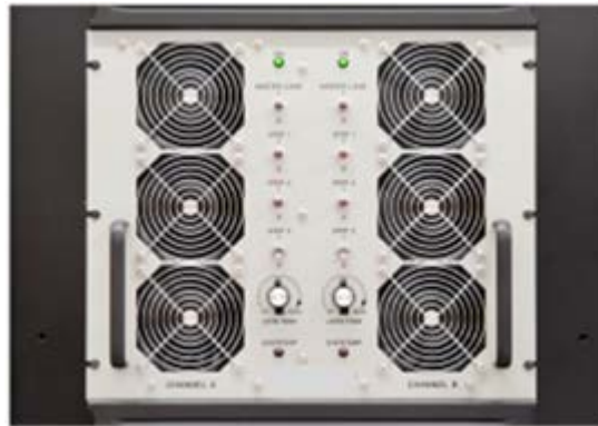
Figure 2. Front panel of 9 RU load bank used for testing.
